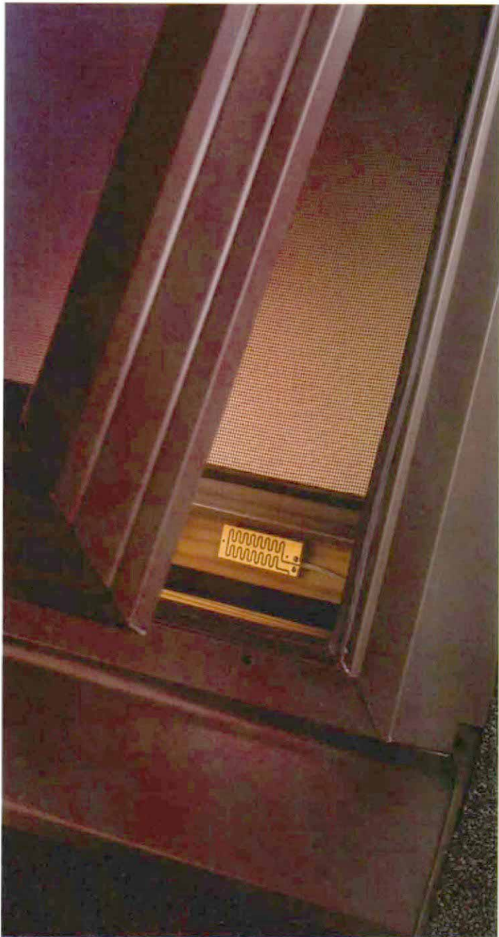
A rain sensor waits for rain. When even a single drop of rain hits this small circuit board, it instantly signals the skylight motor to close the skylight and keep out the rain. Photo courtesy of Velux-America.
