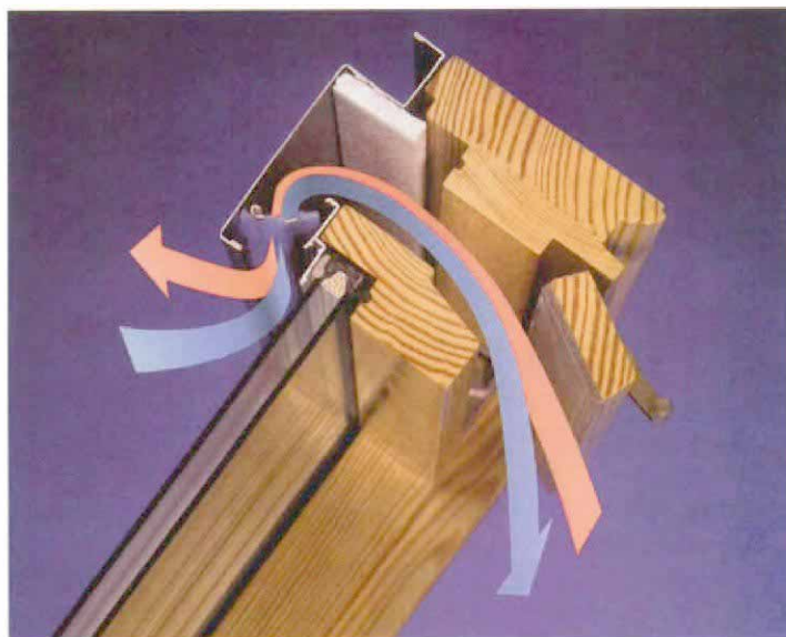
Fixed skylight with ventilation. Velux's FSF skylight does not open, but a ventilation flap at the top lets warm air out and cool air in through a screened channel. Photo courtesy of Velux-America.
